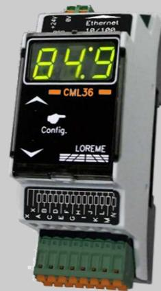
The CML36 is a compact temperature monitoring unit allowing to concentrate up to 32 modules of 14 channels into one Ethernet connection (Modbus TCP protocol) via the internal bus.
