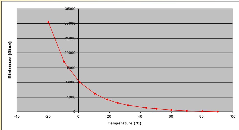
Type "CTN5" (sensitive element **US SENSOR 103JM1A**): With this element, the CML36 measures are not influence by presence of diode.
