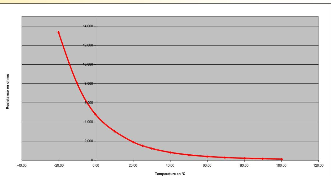
Type "CTN8" (compatible with sensor like "PFEUFFER"): With this element, the CML36 measures are not influence by presence of diode. NTC parameters: Beta = 4000, R0 = 5000 Ohms.
