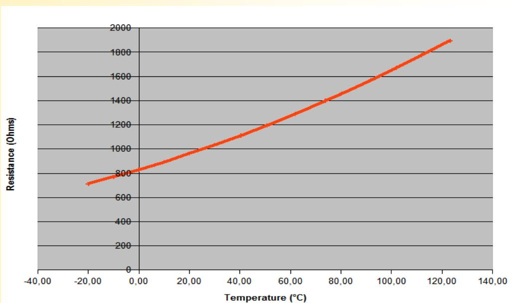
Type "CTN7": With this element, the sensor must not include diode.
