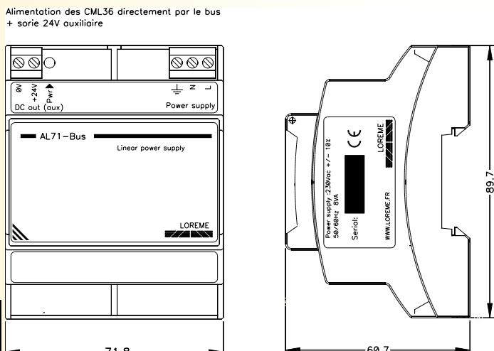
**1 x AL71-BUS + 8 x CML36 maximum.** The power supply can be inserted at any location on the bus
